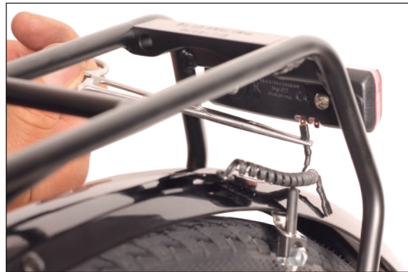
FORCEPS CLAMP useful help for works with lighting cables code 720332
