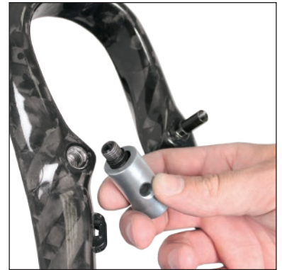
CANTILEVER BOSS EXTRACTOR 9 MM 3/8" drive code 720247
