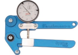
TENSIONAUT-A tensiometer for analog measurement of spoke tension with RADONAUT Art.-Nr. 720351
