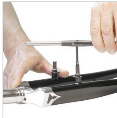
recommended die holder: M5-M6 code 720123 M8-M10 code 720124
