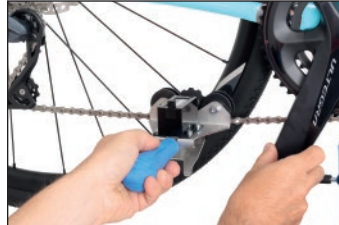
rotate the chain one round
